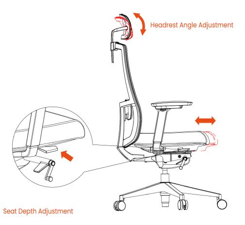
Facing the chair, pull the lever upward with the left hand, hold the right side of the cushion with the right hand, step on the base then pull the seat cushion forward to the proper position.
